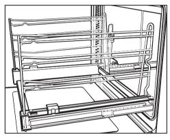
The telescopic baking carriage with 4 levels of runners can be drawn right out of the oven. This gives a good overview of all the cooking in progress.
